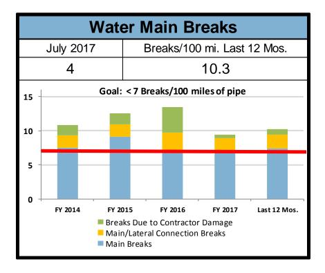
The water main breaks KPI is defined as breaks occurring on water distribution pipes per hundred miles of water distribution pipes.
