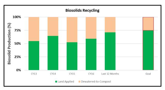
The Biosolids Recycling KPI tracks trends in the amount of biosolids which OWASA applies to land and the amount it dewaters for composting. The WWTP produces an annual average of about 3.5 dry tons of biosolids each day. Most of this is applied in liquid form to agricultural land and a portion is dewatered to the texture and consistency of moist soil and transported to a private composting facility in Chatham County.
